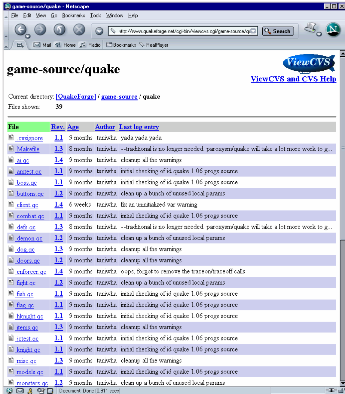
Figure 2. A view into a Web accessible CVS configuration archive of software source code files for the game Quake (source: http://www.quakeforge.net , December 2002).
